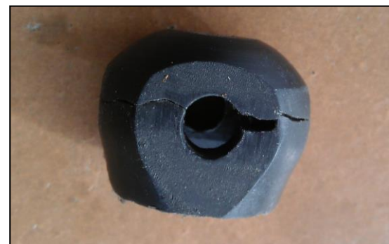
Figure 6: Various failed or excessively loose plastic bushes & balls within brand new aftermarket steering columns
