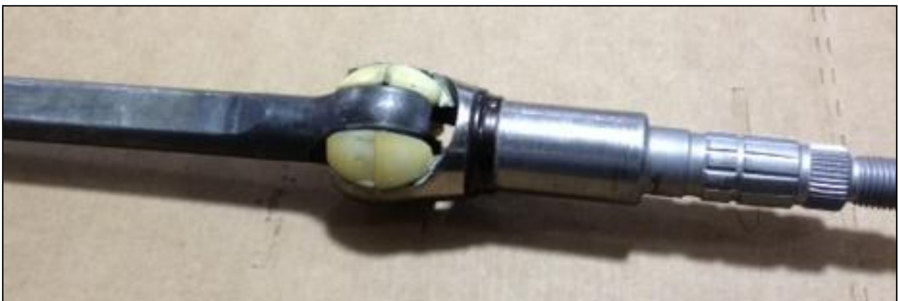
Figure 2: 'GM-style' tilt mechanism assembly, featuring upper and lower yoke shafts
