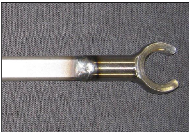
Figure 37: 'Unknown brand B' with GM-style 'double yoke' tilt mechanism, and poor-quality welded connection
