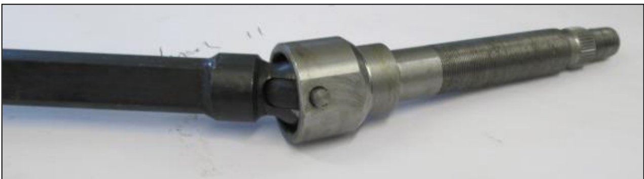
Figure 33: 'Wysco' column with a swivel-joint tilt mechanism
