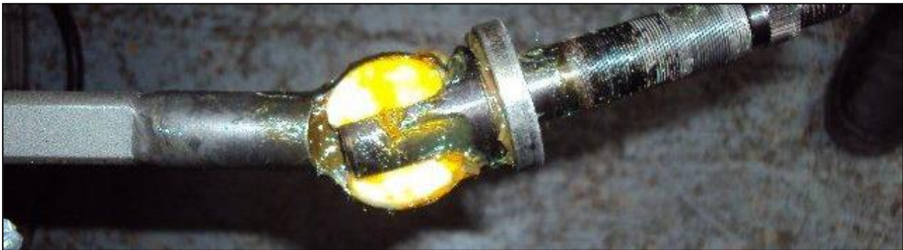
Figure 31: 'RPC' brand uses 'double-yoke' GM-style tilt mechanism
