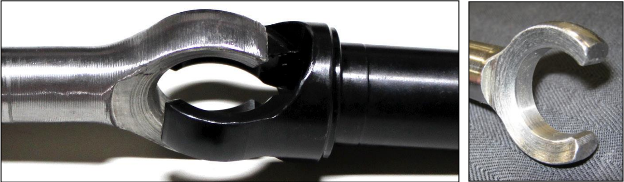
Figure 3: Two 'yokes' of the 'GM-style' tilt mechanism with bush removed, showing 'fail-safe' nature of system
