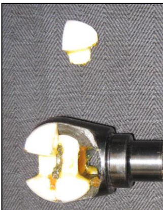
Figure 6: Various failed or excessively loose plastic bushes & balls within brand new aftermarket steering columns
