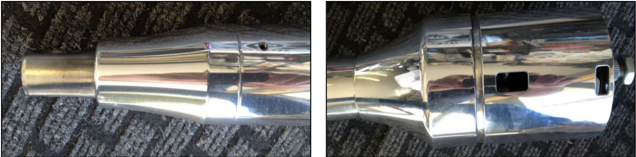
Figure 11: Photographs of tapered base (at left) and shaped upper end (at right) of ‘Billet Specialties’ column
