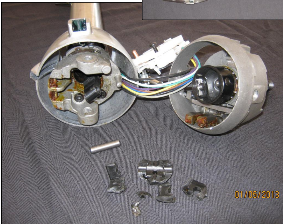
Figure 1: ‘Helix’ brand column, with collapsed plastic tilt mechanism
