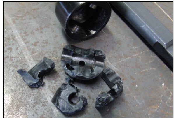
Figure 27: ‘Helix’ column in vehicle at left; collapsed remains of the plastic bush which caused steering failure at right
