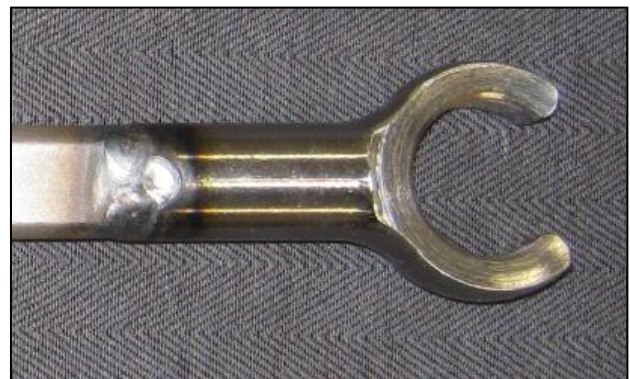
Figure 17: Welded ‘CPP’ yoke-to-shaft connection
