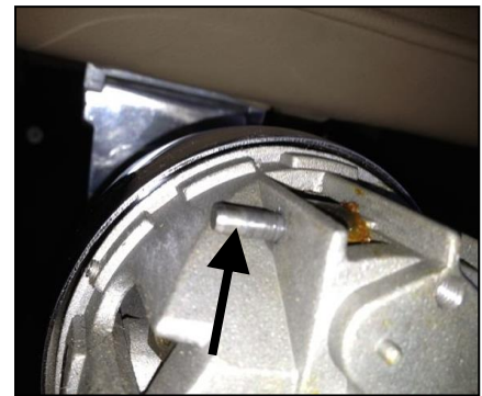
Figure 26: Tilt mechanism pivot lock pin falling out of ‘Helix’ upper housing
