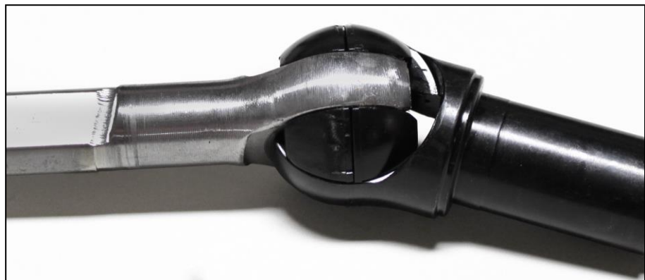
Figure 10: 'Ididit' remanufactured GM-style tilt mechanism & inertia-welded shaft
