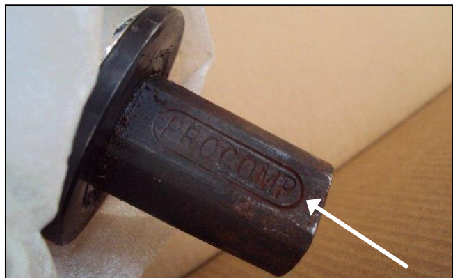
Figure 28: 'Procomp' branding at base of lower column shaft
