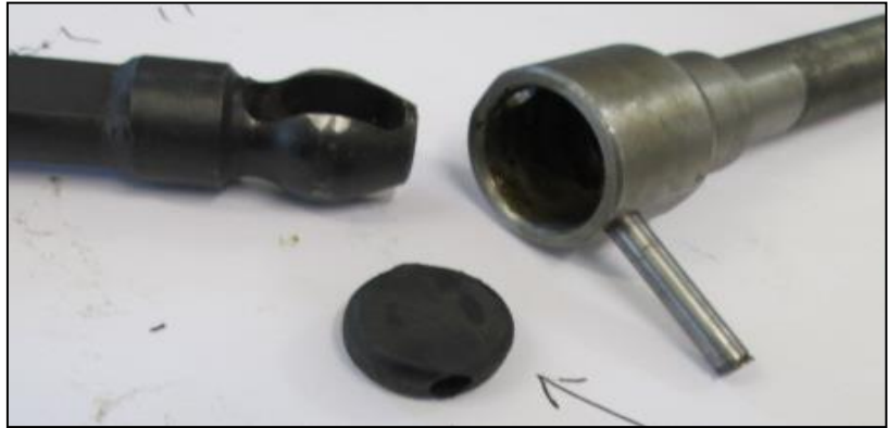
Figure 34: Poor-quality injection-moulded plastic tilt-disc on 'Wysco' column
