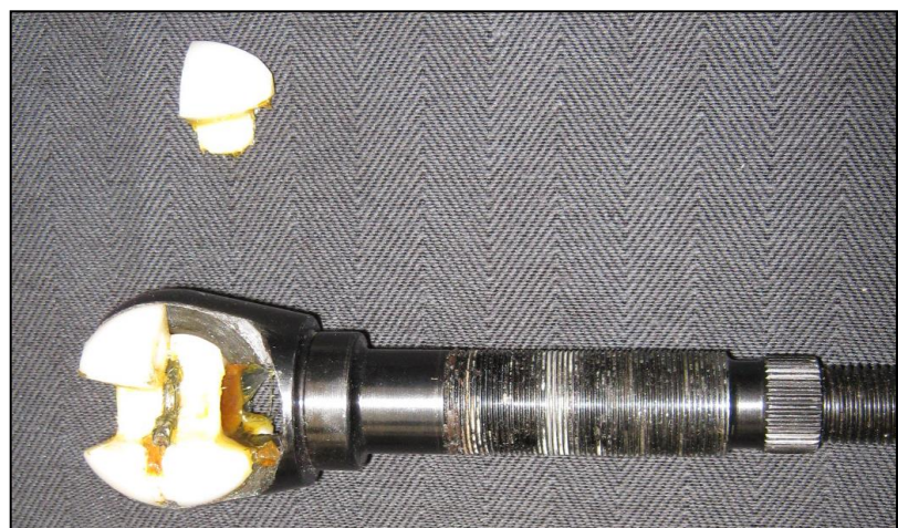
Figure 18: Plastic ball in unused ‘CPP’ column as found during disassembly
