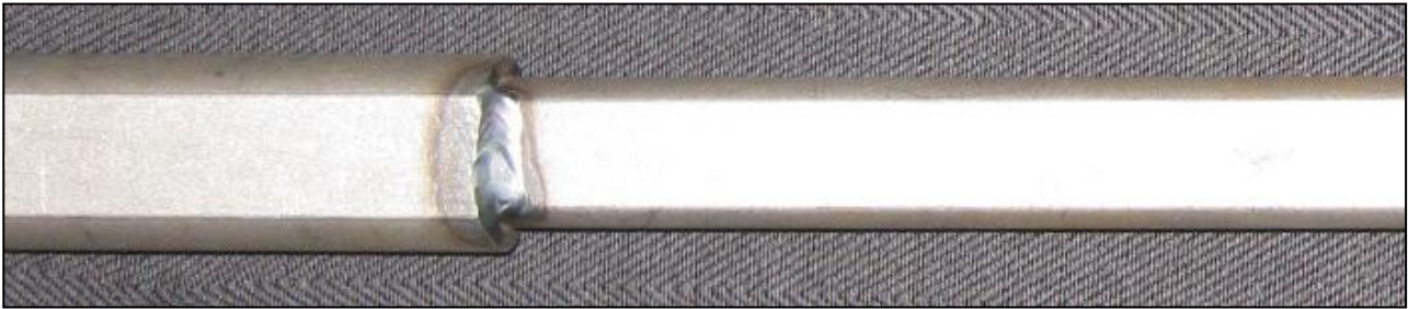
Figure 5: Welding holding two 'double-D' sections together within aftermarket steering column
