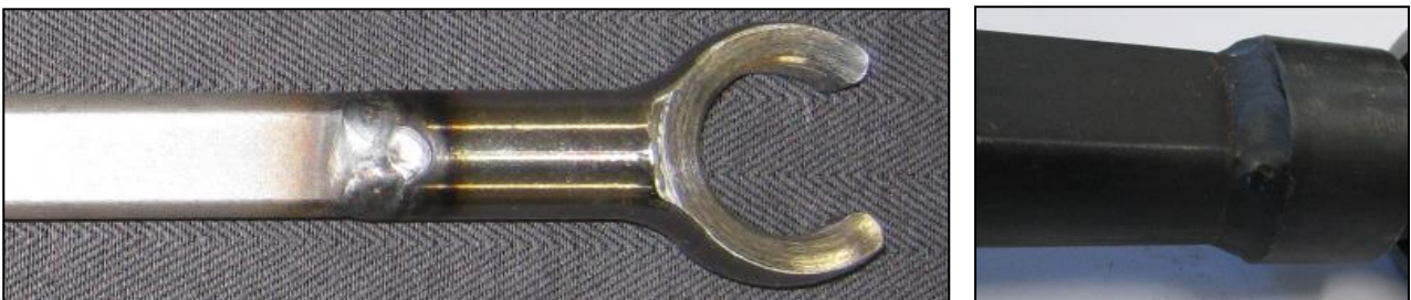
Figure 4: Non-OEM welds within tilt mechanisms in aftermarket steering columns
