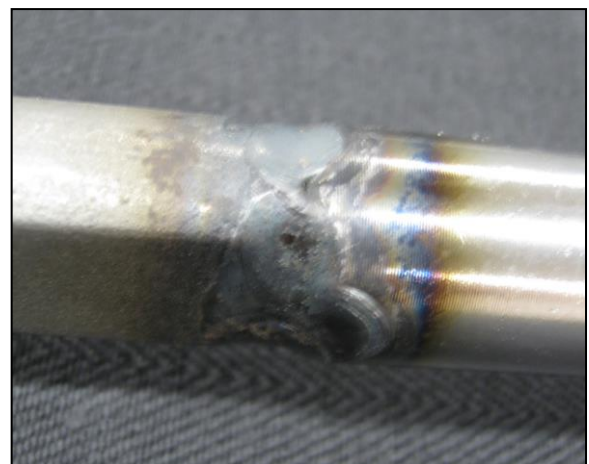
Figure 37: 'Unknown brand B' with GM-style 'double yoke' tilt mechanism, and poor-quality welded connection
