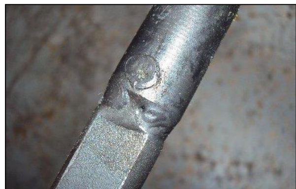
Figure 32: Welded connection in 'RPC' steering shaft
